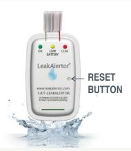
The LeakAlertor that was installed for you is a smart device that electronically monitors your toilet for water wasting problems. When a problem is detected, you will be *alerted both visually and audibly...*
