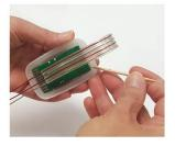
3. Remove the old battery with a toothpick and slide the new battery into place with the "+" side facing UP. (The unit will automatically go into RESET mode.)
